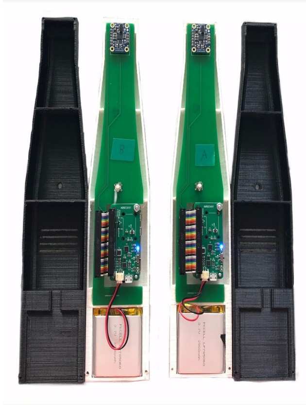
Fig. 8. Close up of the internals of the final design.
