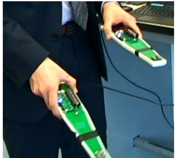
Fig. 7. The drum sticks being operated by Joseph Fitzgerald. The top half of each electronic drumstick were removed for testing and some of the interior components are visible. Near Joe's hand is the Juicebox Zero Power cape connected above the Raspberry Pi. The Raspberry Pi is connected to a set of ribbon wires to a PCB. The PCB contains both a push button (the white dot off of the Juicebox) and the Bno055 (blurry blue component farthest from Joe's hand near the tip of the drumstick).
